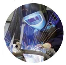
Engineering Tradespersons – Fabrication cut, shape, join and finish metal to make, maintain or repair metal products and structures. They may produce moulds or patterns for metal castings, apply coatings and work with a variety of materials.
