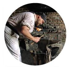
Blacksmiths shape bars, rods and blocks of metal using hand or power tools to produce or repair metal articles. Blacksmiths also make and repair agricultural equipment, mining and quarrying machinery, or ornamental steelwork such as gates and fences. They can specialise in forge-smithing, hammer-smithing or toolsmithing.
