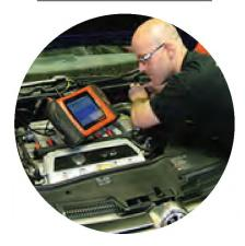
Automotive Electricians install, maintain, identify faults and repair electrical wiring and computer-based equipment in motor vehicles and related equipment, such as caravans, trailers, earthmoving equipment, mining equipment, marine applications and agricultural equipment.
